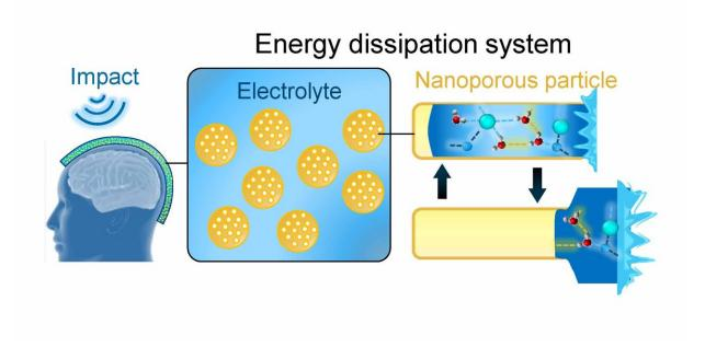
A diagram illustrating how a liquid nanofoam cushion responds to an impact. Credit: B. Xu
