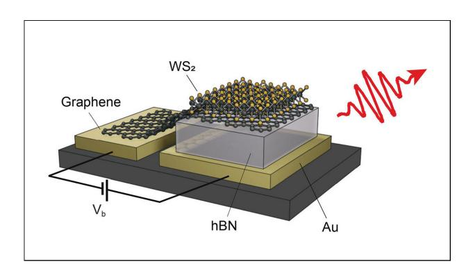
The semiconductor material (tungsten disulfide,  $WS_2$ ) placed outside the tunnel junction (right) acts as an antenna and makes it possible to enhance the energy created in the tunnel junction. Credit: Sotirios Papadopoulos / ETH Zurich
