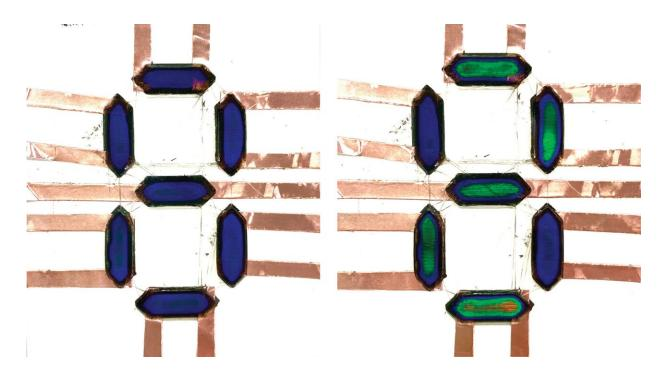
Biodegradable: The display consists of seven electrically conductive segments that change color when a voltage is applied. Credit: Empa
