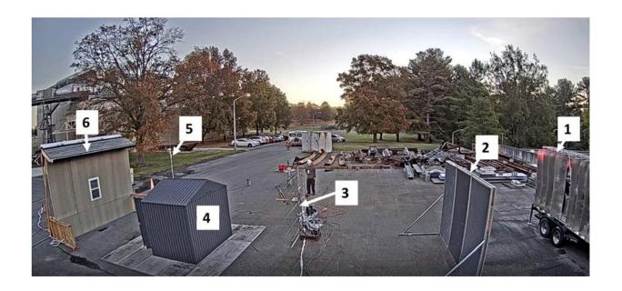
Photograph showing experimental set-up including 1: Wind Machine, 2: Flow Straightener, 3: Array of Bidirectional Probes, 4: Shed, 5: Off-Target Heat Flux Rig, and 6: Target Structure. Credit: *NIST* (2023). DOI: 10.6028/NIST.TN.2253
