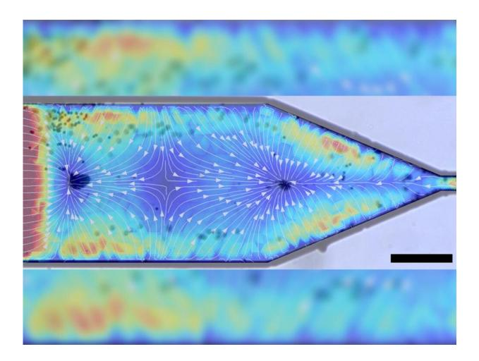
An image of the modeling depicts how the applied ultrasound orients nanorods in a microfluidic nozzle. Credit: Igor Aronson
