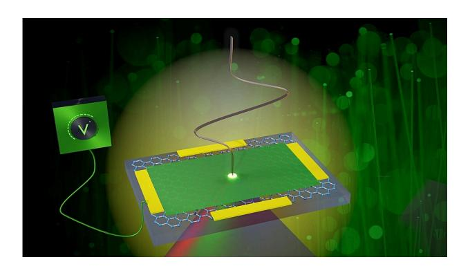
A graphene-based material converts incoming terahertz pulses (from above) into visible light in an ultrafast and controllable manner - optimal for data transport in optical fibers. Credit: B. Schröder/HZDR
