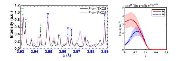
Left: Typical spectral lines measured by the XCS on EAST. Right: The impurity density profiles of  $W^{44+}$ . Credit: Lin Zichao
