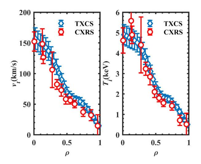
Inverted rotation velocity and ion temperature profiles by XCS compared with Charge Exchange Recombination Spectroscopy (XCRS). Credit: Lin Zichao
