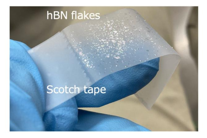
This allowed the researchers to create a thin layer to attach to a target gold wire. Credit: Sasaki et al., 2023
