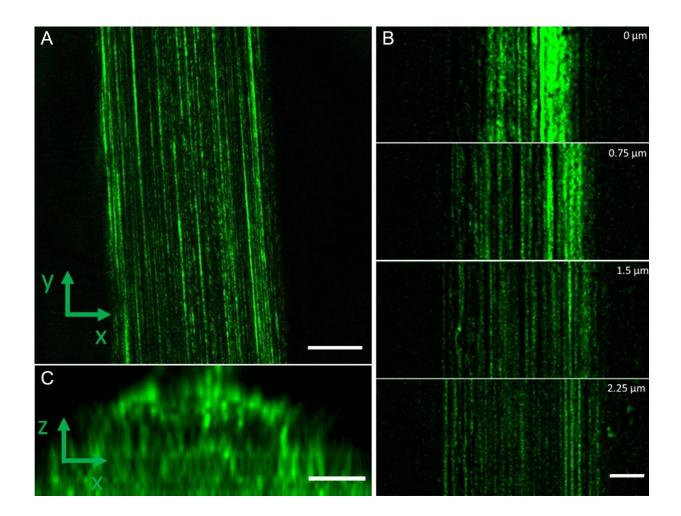
CRFD microscopy images of MAS spider silk fibers (A) Optical slice taken at the middle of a MAS fiber. Scalebar is 5  $\mu$ m. (B) Optical sections of MAS fiber taken at different depths through the fiber. The depth is given by the number in the upper right corner of the images. Scalebar is 2  $\mu$ m (C) Acquisition of images at different depths in z throughout the sample enabled reconstruction of a slice through the fibers in the xz plan, showing the fiber cross section. Scale bars 2
