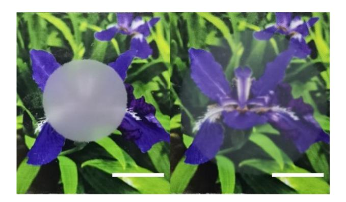
Compressing this soft material blocks a wide range of wavelengths, including visible light (left), and stretching it out lets them through (right). Credit: Adapted from ACS Nano 2023, DOI: 10.1021/acsnano.3c01836
