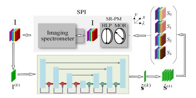
Spectropolarimetric imaging (SPI) scheme for the acquisition of highdimensional 3D data cubes for each Stokes parameter. Credit: *Advanced Photonics Nexus* (2023). DOI: 10.1117/1.APN.2.3.036009
