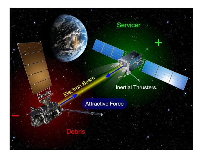
Graphic illustrating how a servicer spacecraft could remove debris from orbit using electrostatic forces. Credit: Schaub Lab
