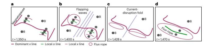
Simplified schematics showing the events within the tail current sheet leading to the eruption of the tail-wide plasmoid. a, The situation within Fig. 1b, showing the two local reconnection regions Earthward and tailward of the dominant x line. Magnetic field topology is given, with  $\odot$  and  $\otimes$  symbols representing outward and inward directions with respect to the plane and corresponding to Bz > 0 and Bz
