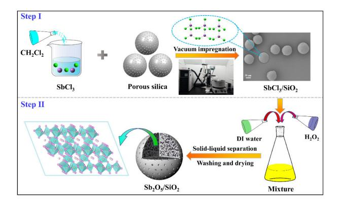
Schematic illustration of  $SbCl_3/SiO_2$  and  $Sb_2O_5/SiO_2$  preparation processes. Credit: Zhang Shichang
