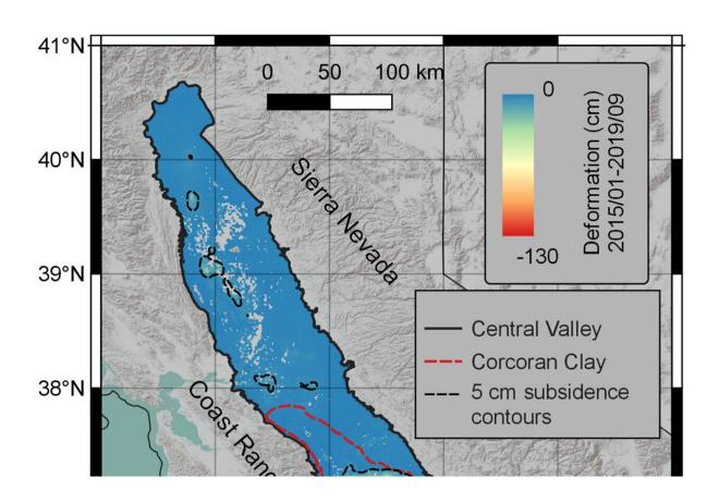
2D map of deformation derived from interferometric synthetic aperture radar data in the Central Valley of California, USA, for the time period 1 January 2015 to 19 September 2019. Credit: *Geophysical Research Letters* (2023). DOI: 10.1029/2023GL103222
