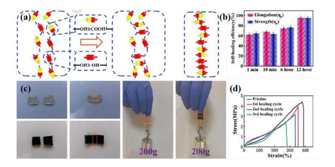
(a) Schematic diagram of self-healing mechanism of hydrogel; (b) self-healing rates 243 of hydrogel at different times; (c)Self-healing demonstration process of hydrogel; (d) 244 Self-healing effect of multiple healing with hydrogel. Credit: Wang et al.
