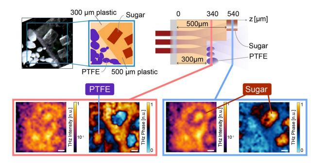
Top left: Photographic image of the cube with objects embedded in it. The popout image is a graphical sketch showing objects made of plastic, sugar and PTFE (a synthetic polymer) embedded at different depths. Top right: A 3D graphical sketch showing terahertz waves passing through the cube. Bottom: Real images captured by the terahertz wave camera. The images show objects embedded in the cube were detected at different depths. Credit: Loughborough University
