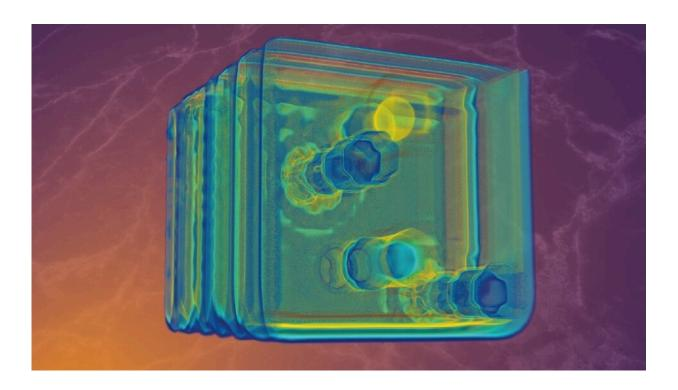
Microscopic, metallic objects distributed throughout a 3D cube. Metallic objects were imaged using the terahertz wave camera and then combined with an artistic, rendered image. Credit: Loughborough University
