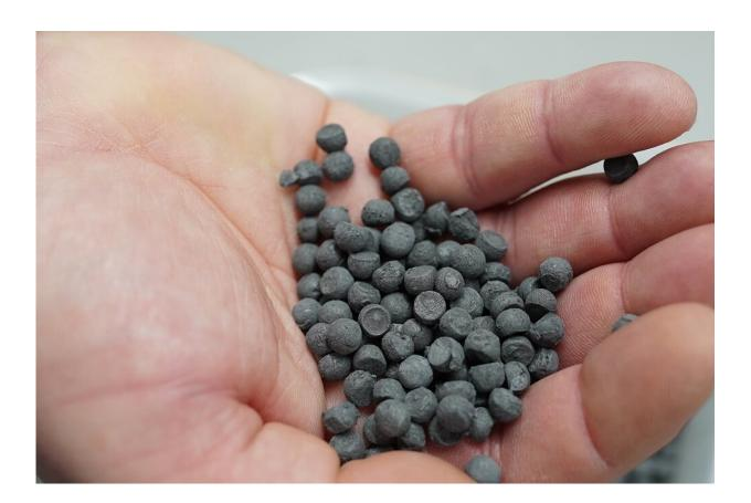
Beads which can store heat, which would otherwise be wasted, from various sources, including industrial operations and the summer sun. The new material has been made using alginate, an inexpensive, abundant and non-toxic seaweed derivative. Credit: SPECIFIC, Swansea University
