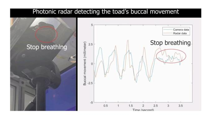
Experimental setup monitoring cane toad breathing in the photonic labs of the University of Sydney Nano Institute. Scientists used a new 'photonic radar' to create high-definition radar to accurately monitor cane toad vital signs. Credit: The University of Sydney
