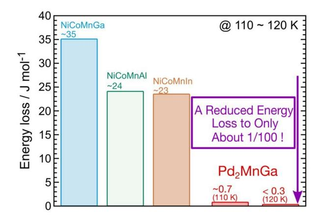
Magnetostriction properties of the current Pd-based alloy at low temperatures. Credit: *Advanced Science* (2023). DOI: 10.1002/advs.202207779
