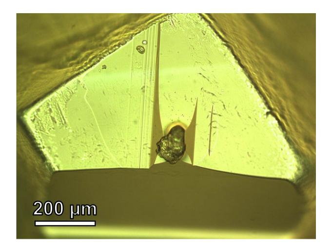
In the lab, Che and Zega embedded the dust particle from asteroid Itokawa in epoxy resin to prepare it for thin sectioning. The scale indicates 200 micrometers, about the width of two or three human hairs placed side by side. Credit: Shaofan Che and Tom Zega / University of Arizona
