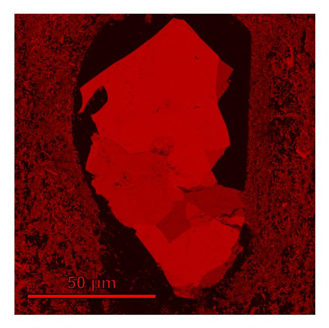
Researchers used a diamond knife to slice through the epoxy and expose a section through the inside of the dust particle, seen here under an electron microscope. Credit: Shaofan Che and Tom Zega / University of Arizona
