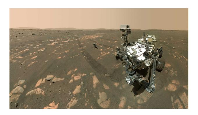
Using the WATSON camera on its robotic arm, NASA's Perseverance Mars rover took a selfie with the Ingenuity helicopter—seen here about 13 feet (3.9 meters) from the rover—on April 6, 2021. Credit: NASA/JPL-Caltech/MSSS
