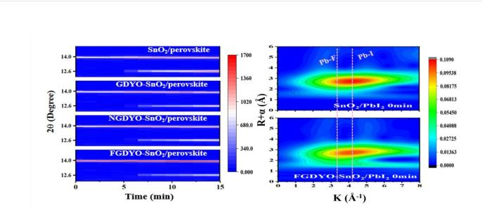
In situ XRD of perovskite on  $SnO_2$  layer with or without GDY-based materials and in situ XAFS spectra of  $PbI_2$  on  $SnO_2$  and  $PbI_2$  on the FGDYO– $SnO_2$  layer. Credit: IHEP
