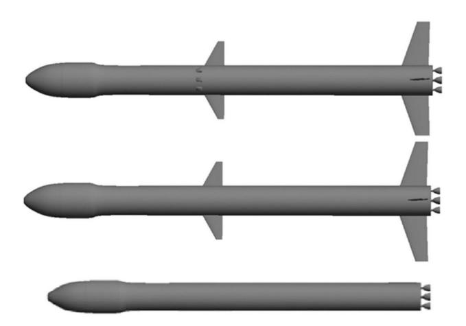
The two architectures (top to bottom), "fly-back" and "glide-back" configurations. Credit: Balesdant, M., et al. (2023)
