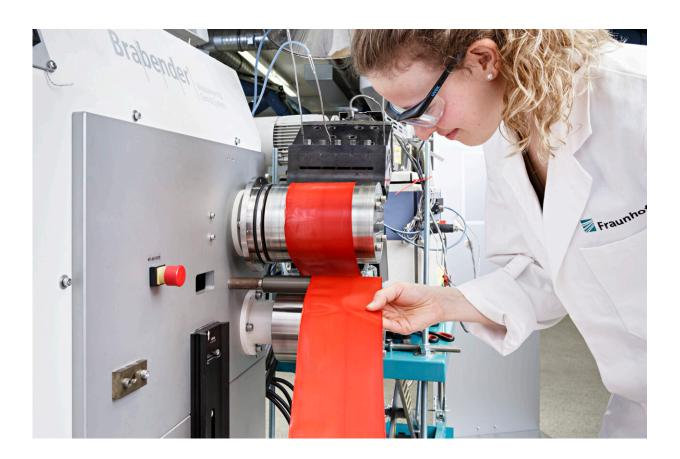
Film processing with a cast film extrusionline. Credit: Ursula Raapke
