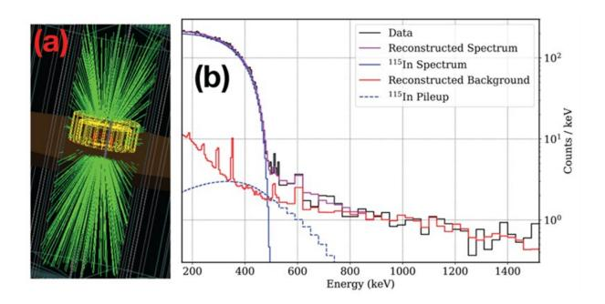
(a) Example simulation showing interactions inside the  $LiInSe_2$  crystal detector . (b) The simulations (red) are combined with expected but mis-reconstructed distribution of events (dashed blue) to extract from data (black) a single In-115 spectrum (solid). Credit: Daniel Mayer/Alexander Leder
