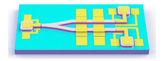
Photonic integration with active—passive functions based on GaN-on-silicon platform. Credit: Jiabin Yan
