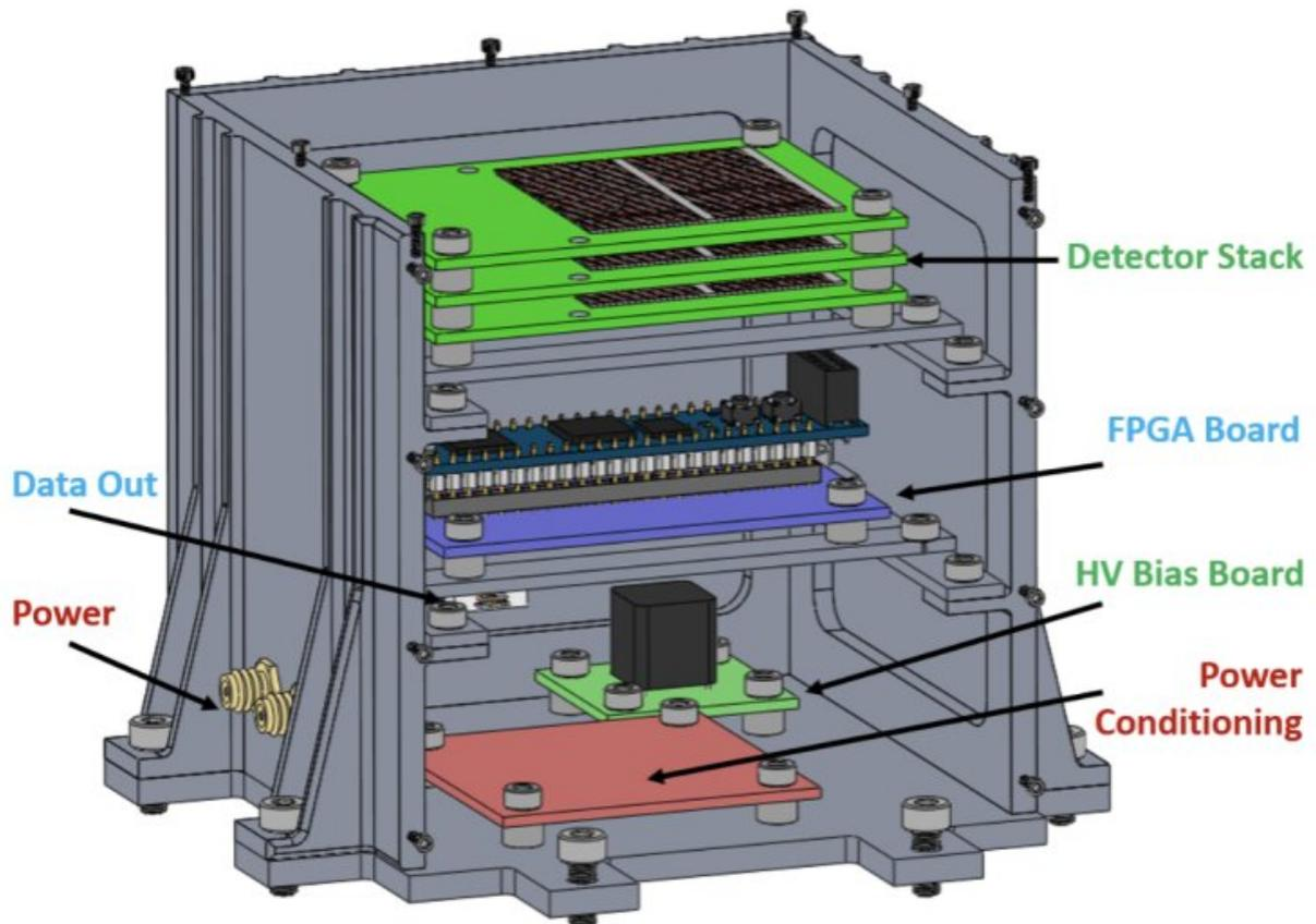
In a practical application like this sounding rocket test instrument design, a gamma-ray observatory would use multiple layers of Astropix sensors, which could then track a 3-dimensional particle trajectory through a series of two-dimensional, pixelated detectors. Credit: Regina Caputo
