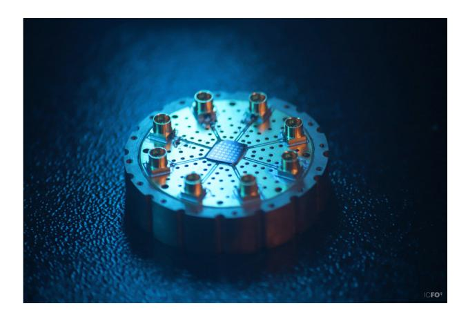
A platform for an array of 36 mechanical resonator devices. Credit: ICFO
