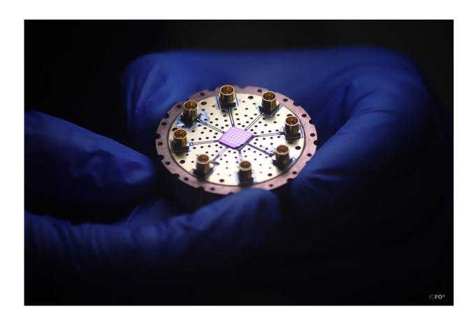
A platform for an array of 36 mechanical resonator devices. A nano-resonator is fabricated and connected electrically in one of the sections of this array. The entire pieces is then placed inside the cryostat for the measurements. Credit: ICFO
