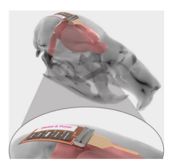
Schematic of the implantable flexible neural probe. Insertion of the flexible neural probe into a rat brain, showing the full system: probe, ZIF connector, and flexible PCB. Resorbable insertion aid covering the flexible neural probe. Credit:
