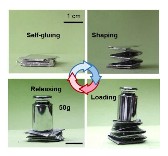
A multifunctional Origami structure built by the liquid metal-treated paper. Credit: *Cell Reports Physical Science*/Yuan et al.
