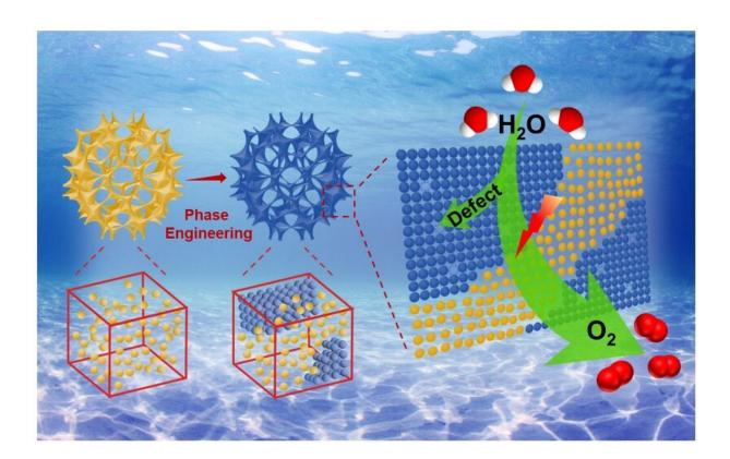
Researchers affiliated with the Beijing Institute of Technology rationally designed an electrocatalyst with both amorphous and crystalline phases, as well as abundant defects, to more efficiently split water and produce clean-burning hydrogen gas. Credit: Nano Research Energy, Tsinghua University Press
