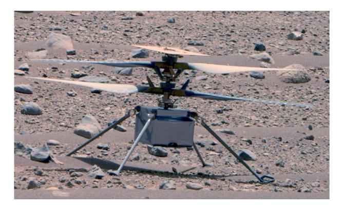
NASA's Ingenuity Mars Helicopter was captured by the Perseverance rover's Mastcam-Z on April 16, not long after the rotorcraft's 50th flight. The helicopter would soon fall silent for 63 days due hilly terrain that interrupted communications between the rover and aircraft. Credit: NASA/JPL-Caltech/ASU/MSSS
