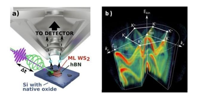
Left, ultrafast light pulses excite and probe a tiny sample of WS2 one layer of atoms thick, emitting electrons that are collected by a new detector called a momentum microscope. Right, full 3-D energy-momentum distribution of the emitted electrons. Credit: Stony Brook University
