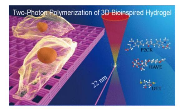
Schematic illustration of TPP of HAVE 3D hydrogel structures. Credit: Zheng et al
