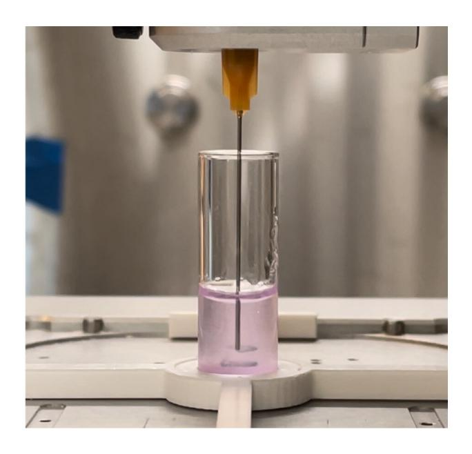
Extrusion bioprinting within a granulated gel. Credit: Advanced Materials (2023).
