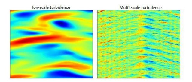
The contrast between turbulence driven by large-scale ion motion (left) and multiscale turbulence that couples with the fast, small-scale motion of electrons (right) to drive heat loss in a tokamak. Credit: E.A. Belli
