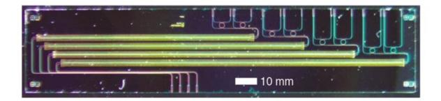
Optical micrograph of the electro-optic isolator chip on thin-film lithium niobate, comprising four devices with varying modulation length. Credit: Loncar Lab/Harvard SEAS
