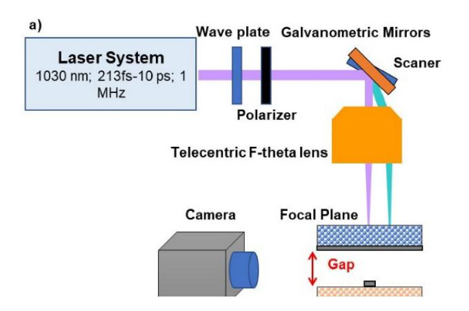
a) Schematic of the experimental system used in polymer printing. It includes a laser with a variable pulse duration between 210 fs and 10 ps, a wavelength of 1030 nm and a repetition frequency of up to 1 MHz. In addition, it includes a scanner and an F-theta lens that allows you to move the position of the focus of the laser along a  $5 \times 5$  cm<sup>2</sup> surface. b) Schematic of the printing process. Credit: Optics Express (2023). DOI: 10.1364/OE.488859
