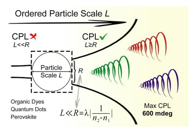
A schematic diagram of the scale-effect model based on scalar theory. Credit: Science China Press
