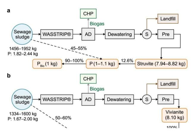
Three P recovery pathways were assessed starting from sewage sludge, all of which included assessments of anaerobic digestion (AD), combined heat and power (CHP), dewatering, and solid–liquid separation. Credit: The authors
