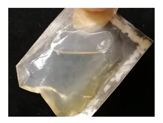
By incorporating soy protein into the structure and coating it with an oil-resistant composite, the CUHK team successfully created an edible, transparent, and robust BC-based composite packaging. Credit: To Ngai
