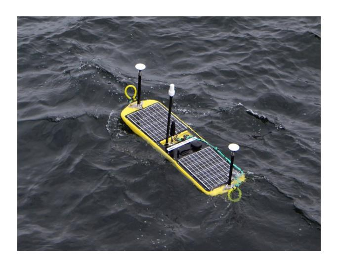
A wave glider with GNSS and acoustic measuring devices for measurements on the seafloor. Credit: Todd Ericksen
