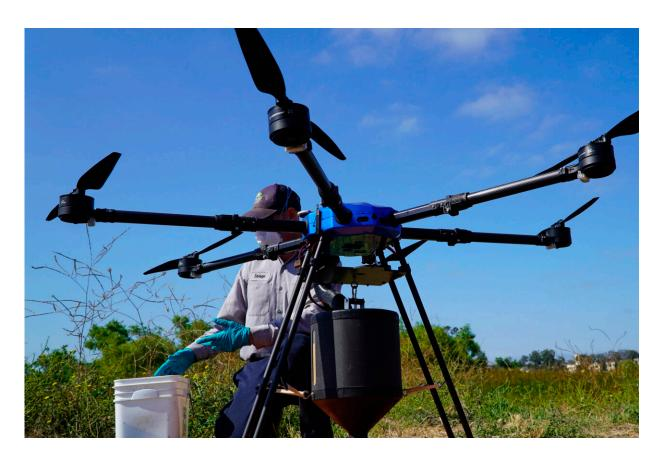
Drone pilot John Savage loads a hexacopter drone with anti-mosquito bacterial spore pellets at the San Joaquin Marsh Reserve at University of California in Irvine, Calif., on June 27, 2023. The drone is the latest technology deployed by the Orange County Mosquito and Vector Control District to attack mosquitoes developing in marshes, wetlands, large ponds and parks. Credit: AP Photo/Eugene Garcia
