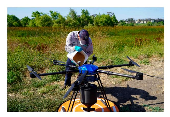
Drone pilot John Savage loads the hexacopter drone with anti-mosquito bacterial spore pellets at the San Joaquin Marsh Reserve at University of California in Irvine, Calif., on June 27, 2023. The drone is the latest technology deployed by the Orange County Mosquito and Vector Control District to attack mosquitoes developing in marshes, wetlands, large ponds and parks. Credit: AP Photo/Eugene Garcia
