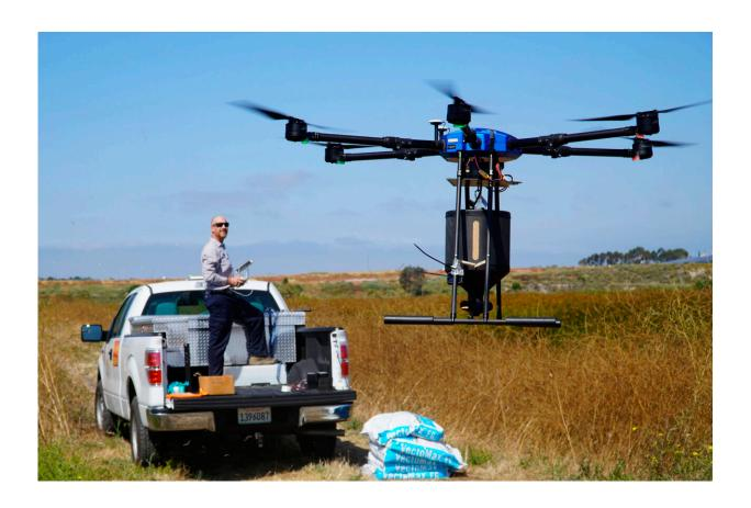
Drone pilot John Savage flies the hexacopter drone loaded with anti-mosquito bacterial spore pellets at the San Joaquin Marsh Reserve at University of California in Irvine, Calif., on June 27, 2023. The drone is the latest technology deployed by the Orange County Mosquito and Vector Control District to attack mosquitoes developing in marshes, wetlands, large ponds and parks. Credit: AP Photo/Eugene Garcia
