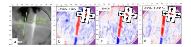
a) XAS of the device, with the magnetic field in the direction of the nanowire but with the X-ray beam in the direction of the contact wire. b-d) XMCD in the same configuration. With this configuration the magnetization of the contact can be probed. These measurements together with the ones in Figure 2 allows to unequivocally define the magnetization direction in our device. Credit: *Advanced Materials* (2023). DOI: 10.1002/adma.202211176
