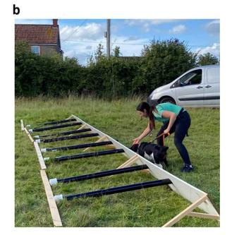
Channeled distance perception rig setup. (a) Channeled distance perception rig setup viewed from the front. For details see text. (b) View of the rig from the back with detection dog Freya and handler Nikki Glover moving along front of the rig checking each pipe entrance. Credit: Glover et al, 2023, *PLOS ONE*, CC-BY 4.0 (creativecommons.org/licenses/by/4.0/)
