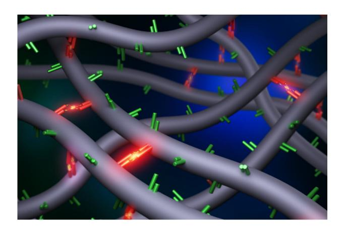
A 3D rendering illustrating two monomers forming a reversible double-hydrogen bond that slows down polymer movement without creating an elastic network. Selected for a Synopsis in Physics and an Editors' Suggestion, and highlighted as the front cover in Physical Review Letters. Credit: S. Nian et al., *Phys. Rev. Lett.* 130, 228101 (2023)
