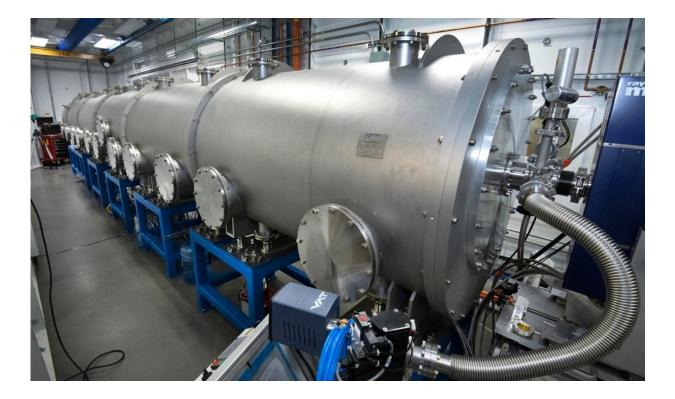
Cai's collaborators at the National Synchrotron Light Source II conducted experiments using a sophisticated X-ray tool — the soft matter interfaces beamline shown here — to reveal the inner makeup of the polymers without damaging the samples. Credit: University of Virginia
