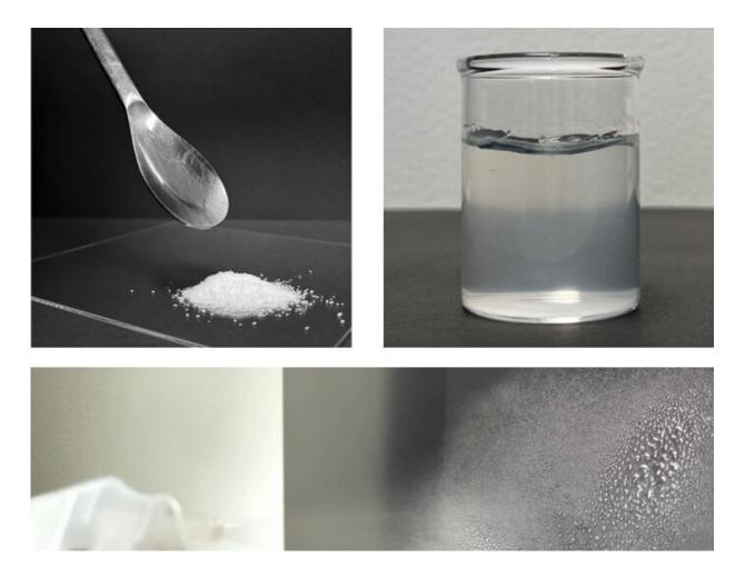
Evaporated CNF powders have a small volume and no handling issues related to static electricity (upper left). Their water dispersions are colorless and transparent (upper right) and dispersion droplets formed by spraying do not drip (lower). Credit: 2023 Nogi et al., Evaporative Dry Powders Derived From Cellulose Nanofiber Organogels to Fully Recover Inherent High Viscosity and High Transparency of Water Dispersion. Macromolecular Rapid Communications
