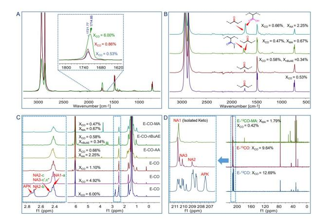
A: IR spectra of E/CO copolymers; B: IR spectra of E/CO/PM terpolymers; C: 1H NMR spectra of copolymers and terpolymers; D: 13C NMR spectra of 13CO-
