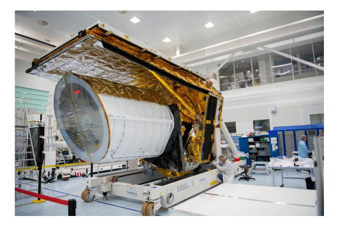
Structural and thermal model of the Euclid satellite. Credit: ESA–S. Corvaja
